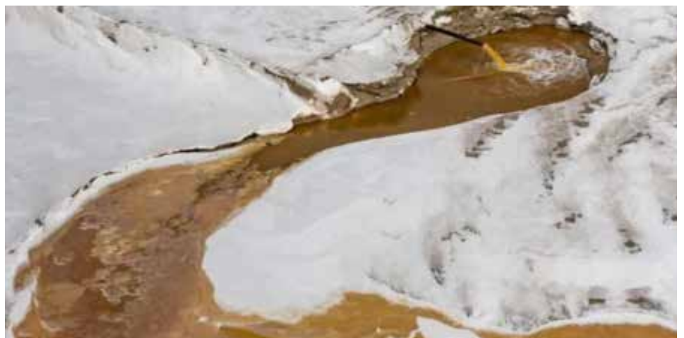
Pictured above is a typical tailings stream being deposited into a tailings pond.
